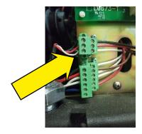
• Make sure Switch 2 is OFF on the I/O board in the HA33 customer unit.
